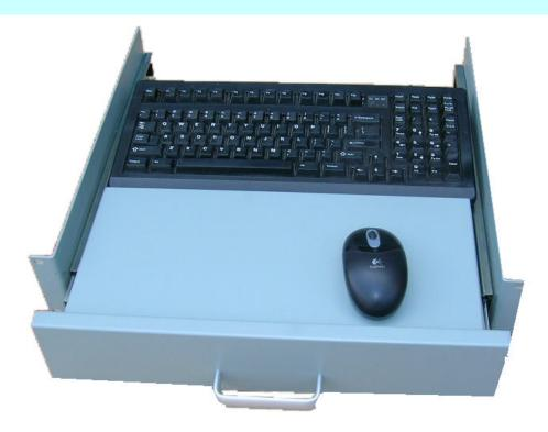
This slide keyboard shelf can hold a standard keyboard with width under 17" and height up to 1.5". The top of hinged cover for storage compartment serves as writing shelf, arm rest, or mounse pad. A cable holdong bar is designed for secure keyboard and mouse cables. An adhesive hook and loop is provided for holding the keyboard in place. This shelf requires 3.5" of panel space (2RU) and 16" depth. Use P/N 15-2403Kx for 24" racks. Please use our standard color code for suffix – x.
