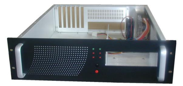
This is a spacer saver model for rack mount PC which requires no raiser card. All cables and wires are connected in the back of the chassis. One CD-ROM opening and 2 internal HDD spaces are available. Motherboard sits on a universal mounting plate for easy removal. A 12VDC fan is mounted behind front panel with filter to intake air and to pressurize inside to prevent dust entering. Additional fan for CPU is included.
