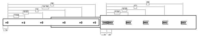
These 3-section ball bearing steel slides have full extension with quick disconnect function. They will fit into 1RU space, and can handle a full load rating of 100 lbs. per pair. A set of 4 mounting brackets and screws (16 of the 8-32 thread) are included. Standard finish is electro zinc plated. Other travel lengths and finish also available.
